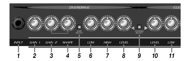
**1: INPUT:** Connect your guitar here using a shielded instrument cable.
